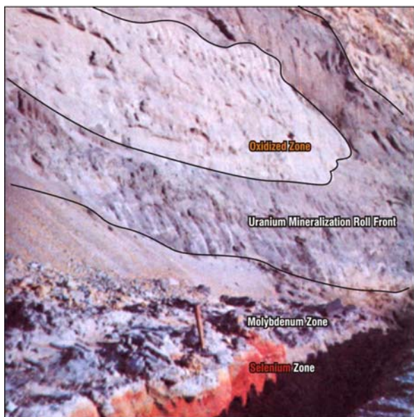
Figure 5. Pit wall of uranium roll-front (geochemical cell) (after Dickinson and Duval, 1977).
