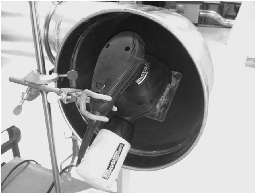
Fig. 4 The sander at the inlet to the duct
