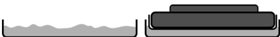
Fig. 1 Illustration of powder placement in the incubation experiments where the left - and right -hand image shows the petri dish for pure humidity and combined humidity–pressure load incubations, respectively
