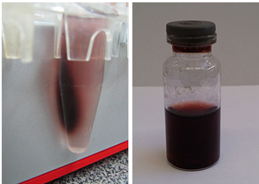
Fig. 10 Digital images of solution of \text{polymer@Au}/\text{Fe}_3\text{O}_4 nanoparticles, dispersion of magnetic nanoparticles, and magnetic response of nanoparticles (right to left)
