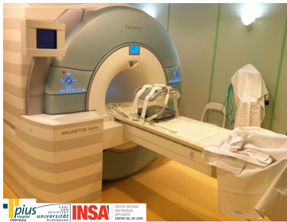
Fig. 18 The clinical Siemens Magnetom Verio 3T MRI scanner with the square acrylic box filled with water that contains bolus of aggregates
