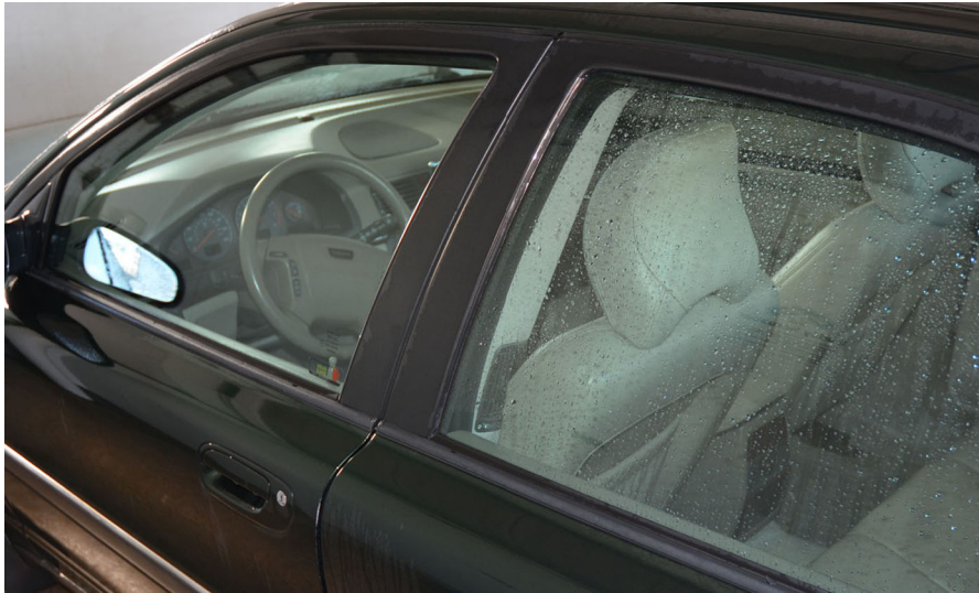
Fig. 8 Demonstration of wetting behavior: Driver's seat window was coated with nanoparticles, while rear passenger window was uncoated. When water was sprayed on both of the
