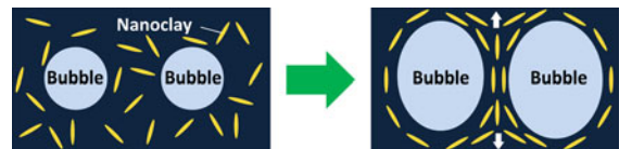
Fig. 10 Alignment of nanoclay particles during bubble growth
