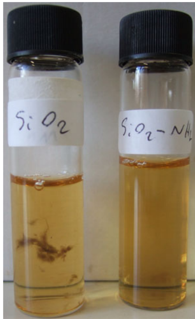
Fig. 4 Silica-coated IONP (left), surface functionalized silica-coated IONP (right) after 1 week dispersion in pure water
