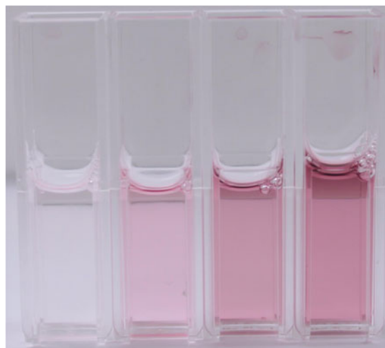
Fig. 2 Color of RT60, RT70, RT80, and RT90 samples (from left to right, respectively) after heating at 70 °C for 3 min. (Color figure online)
