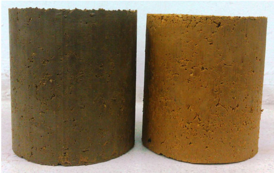
Fig. 3 Color of soil samples after compaction, the sample with light color is S3 and the sample with dark color is S3 with 0.5 % nano-copper
