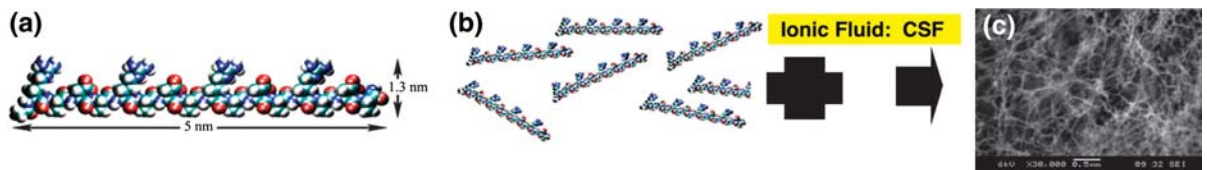
Fig. 41 Small self-complementary 16-residue polypeptide nanoelements that organize into “self-assembled peptide nanofiber scaffoldings” (SAPNS) and exhibit substantive adhesion to
