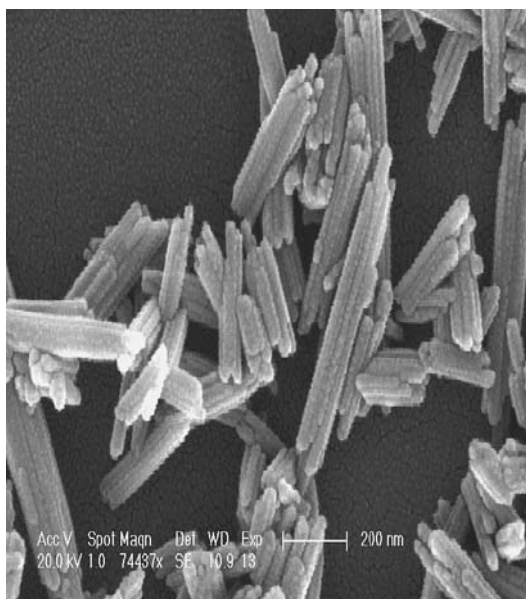
Figure 5. ESEM images of the \text{Sm}(\text{OH})_3 nanobundles.
