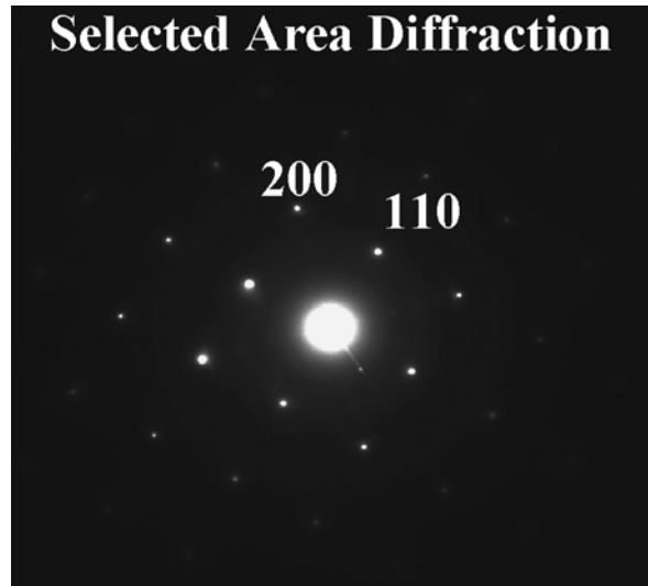
Figure 4. E-beam diffraction pattern on the core of clusters, which shows Fe BCC structure.
