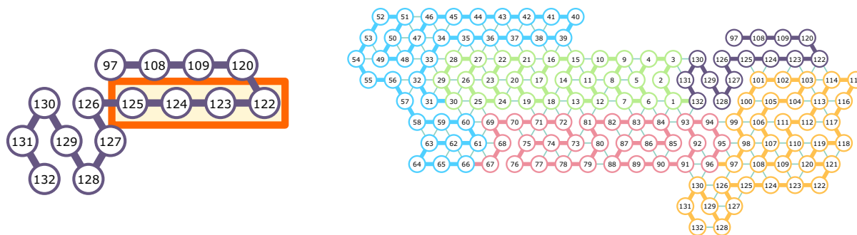
Fig. 13 Counting from a non-coding seed. (Left) The simplest-possible seed that consists only of the boxed right Turn Signal. (Right) Starting from this non-coding seed, the first period results in the counter value 1 in the 1-bit
