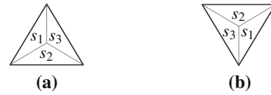
Fig. 4 a An up-triangle cell, and b a down-triangle cell in the space of ETPCA, whose states are (s_1, s_2, s_3) \in \{0, 1\}^3
