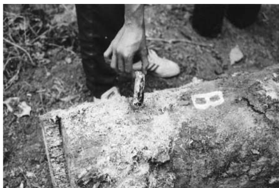
Figure 1. Dowels were inserted into the oil palm tissues at 0.5 m intervals along the length of the trunk and at intervals around the circumference.
