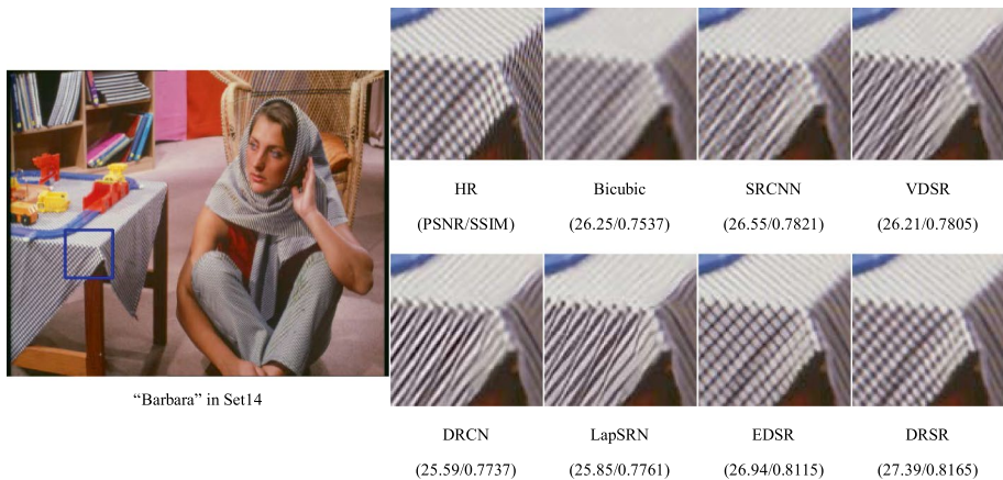
Fig. 7 Qualitative comparisons of DRSR and other models with scale \times 3 using image “Barbara” on Set14
