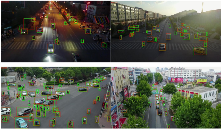
Fig. 6 Visualization of our detection results on the VisDrone validation set. We denote ground truth in green and detection results in red (Color figure online)
