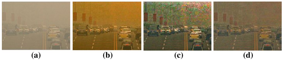
Fig. 2 The performance of dehazing algorithms on the dust haze image. a Dust haze image. b He et al.'s method. c Meng et al.'s method. d Huang et al.'s method
