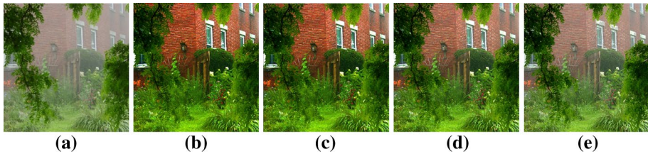
Fig. 6 Restored image with different \sigma . a Original image. b \sigma=0.1 . c \sigma=0.3 . d \sigma=0.5 . e \sigma=0.8
