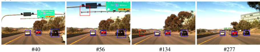
Fig. 12 Sample qualitative results for the proposed method on LISA 2010 dataset, such that (a) Highway-dense sequence, (b) Highway-medium or sunny sequence: (blue) true positive, and (red) false positive (Color figure online)
