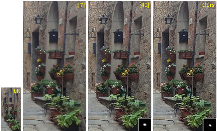
Fig. 14 Super-resolution with a realistic LR image (Flower, the up-sampling factor is 3). Left to right: LR image, non-blind ANR (Levin et al. 2011b), Michaeli and Irani (2013), and our proposed method
