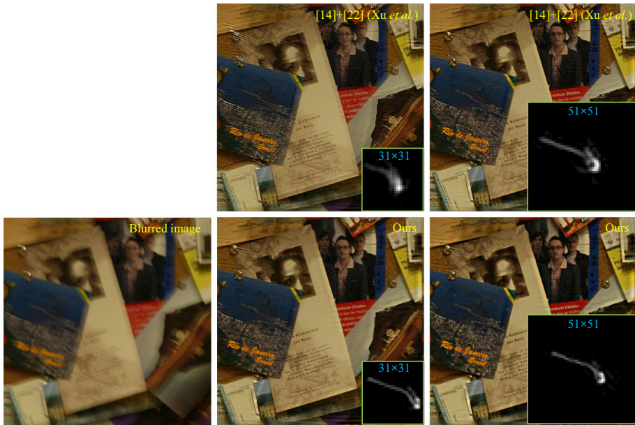
Fig. 8 Blind deblurring results by our method and (Xu et al. 2013; Dong et al. 2014) assuming two kernel sizes. Note that in our method, \alpha_0 is set as 0.15
