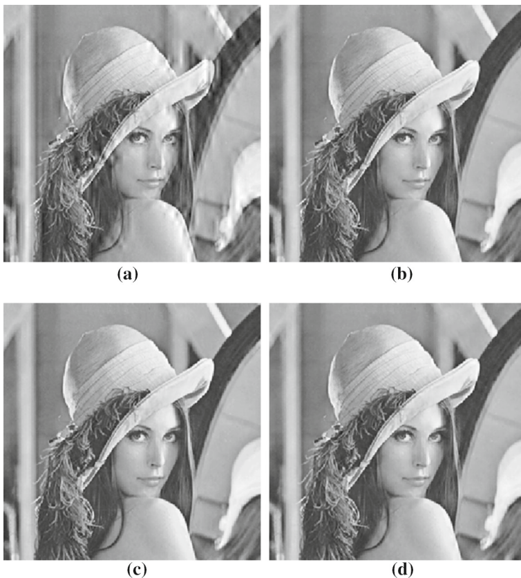
Fig. 11 Whole LH subband ( 32 \times 32 ) loss a received image, b the result by FOTV-PD ( \alpha = 1.2 , PSNR = 33.36 dB, CPU time = 15.46 s), c restored image by TV-PD (PSNR = 30.92 dB, CPU time = 13.39 s), d restored image by NLTV-BOS (PSNR = 31.33 dB, CPU time = 500.23 s)
