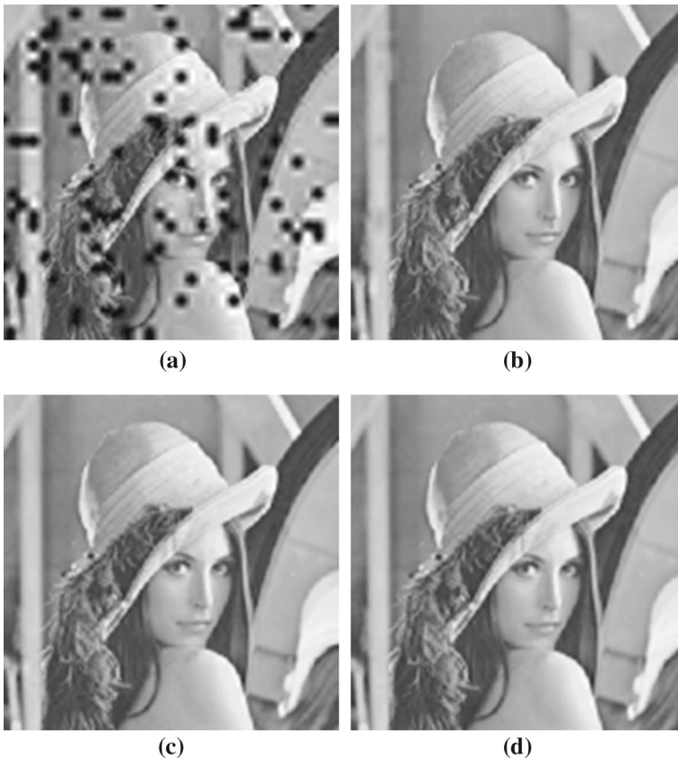
Fig. 4 The Lena image with 10% of wavelet coefficients lost: a received image, b restored image with \alpha = 0.8 (PSNR = 32.28 dB), c restored image with \alpha = 1.2 (PSNR = 33.45 dB), d restored image with \alpha = 1.4 (PSNR = 34.86 dB)
