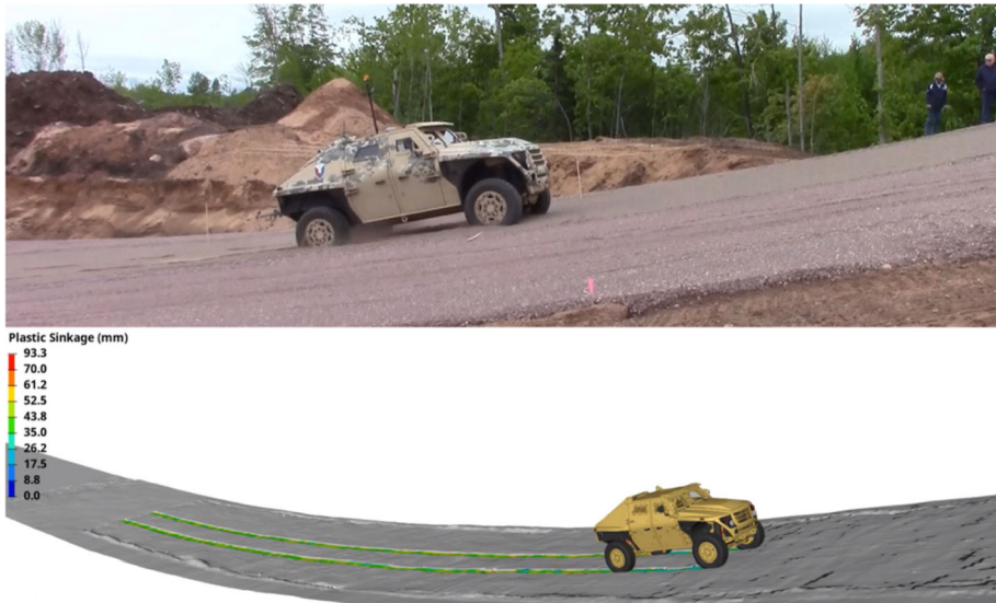
Fig. 18 Variable slope climbing maneuver: Terrain surface and resulting soil plastic sinkage
