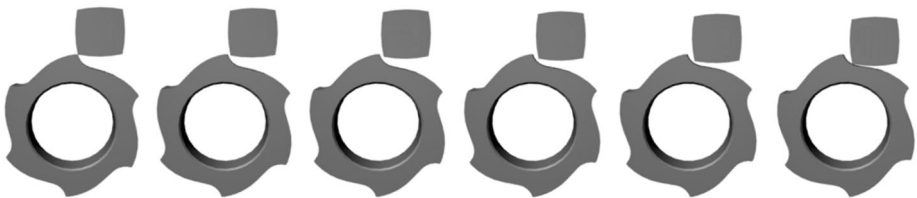
Fig. 19 Animation sequence of the virtual simulation of the cam-follower movement during the first instants after the follower reaches the up dead point
