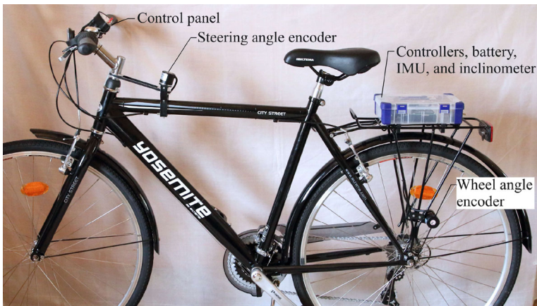
Fig. 3 Overview of the instrumented bicycle
