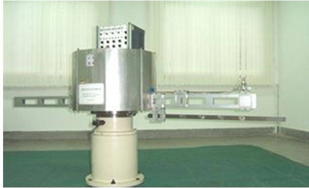
Fig. 11 Air floating platform undergoing rotational motion
