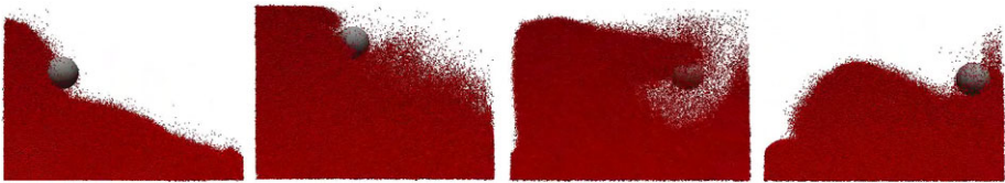
Fig. 2 Light ball floating on 1 million rigid bodies moving around in a tank while interacting through friction and contact. The simulation setup is discussed in [3]; the parallel implementation of the dynamics solution is presented in [2]. The collision detection stage found on average more than 3 million contacts at each time step of the simulation
