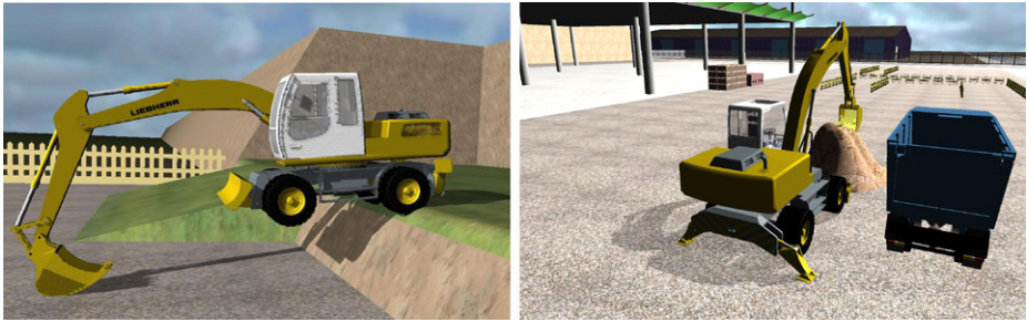
Fig. 10 Using the arm for descending a steep slope and terrain excavation
