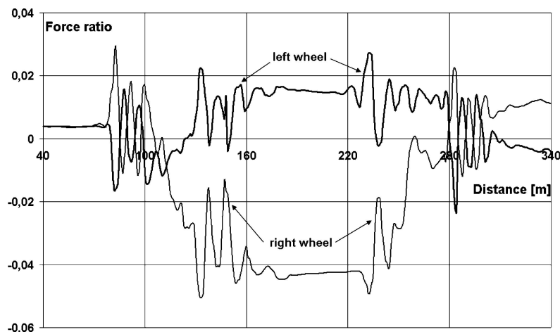
Figure 12. Lateral to vertical forces ratio on the front bogie wheels.
