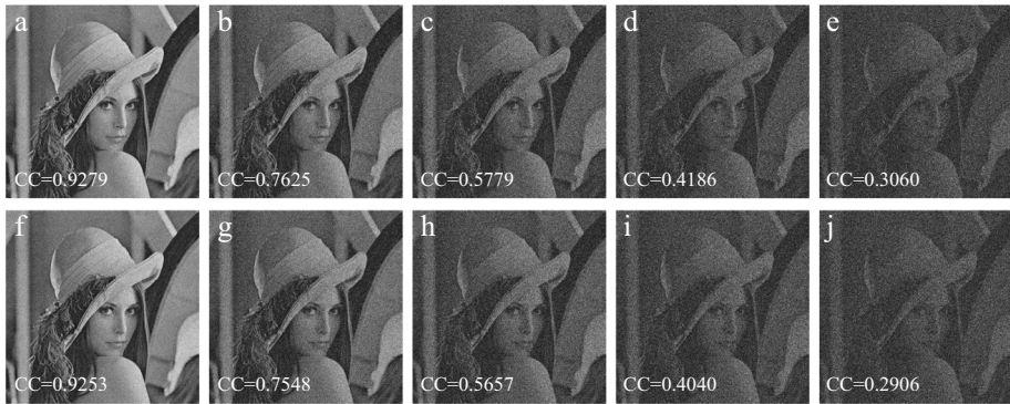
Fig. 15 Decrypted images from contaminated first ciphertext by Gaussian noises with different noise strengths b : (a) 0.2, (b) 0.4, (c) 0.6, (d) 0.8, (e) 1.0, respectively; decrypted images from contaminated second ciphertext by Gaussian noises with different noise strengths b : (f) 0.2, (g) 0.4, (h) 0.6, (i) 0.8, (j) 1.0, respectively
