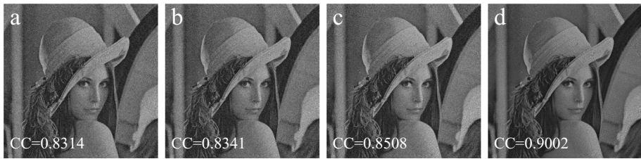
Fig. 11 (a)-(d) Decrypted image of the 3D-SPEA using wrong key with the rotation angle deviation \Delta\beta_n (n = 1, 2, 3, 4) of 10^{-3} , respectively
