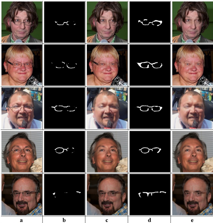
Fig. 7 Mask completion impact on eyeglass removal. (a) Images with eyeglasses or inputs, (b) Predicted mask by E&S-R Method, (c) Generated images of eyeglass removal by E&S-R, (d) Mask completion by proposed method and (e) Generated images of eyeglass removal by the proposed method
