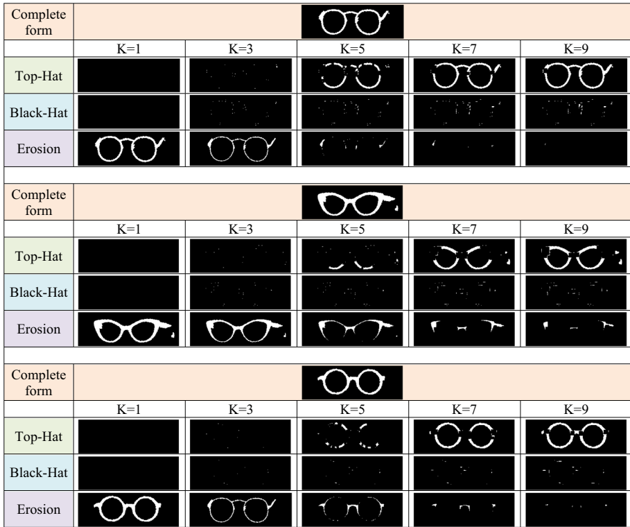
Fig. 8 Effect of different morphological transformations: Top-Hat, Black-Hat, and Erosion (odd kernels 1–9) on the complete form of eyeglasses masks
