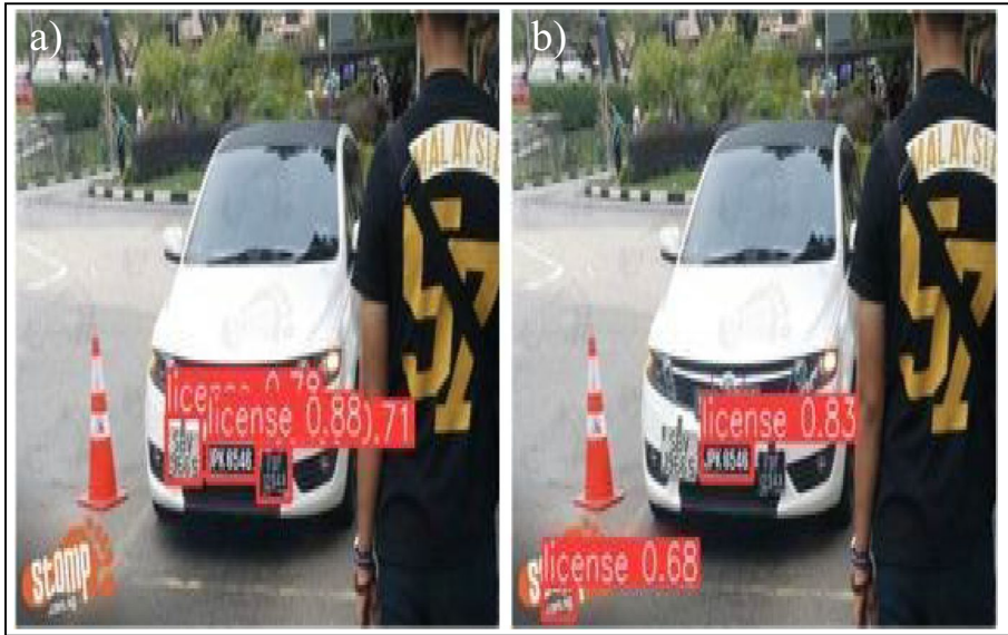
Fig. 10 a LPs detected with 2 Augmentation Model. b LPs detected with 1 Augmentation Model
