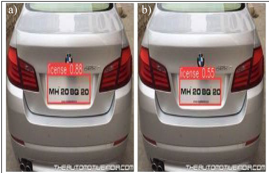
Fig. 11 Ideal scenario (back facing car) (a) 2 Augmentation model; b 1 Augmentation confidence about the detection of LP
