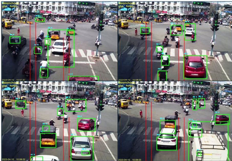
Fig. 13 Displacement of an object within N=4 frames
