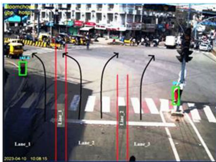
(a) Traffic Rules Defined at Traffic Junction
