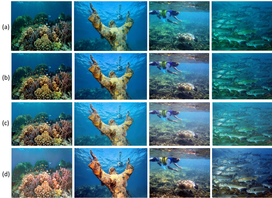
Fig. 8 Enhancement results of CAViT and CAViT G trained on LUSI. (a): Input images. (b): Enhanced results using the model trained on Train-L. (c): Enhanced results using the model trained with the Gamma Correction component on Train-L. (d): Reference images (recognized as ground truth (GT))
