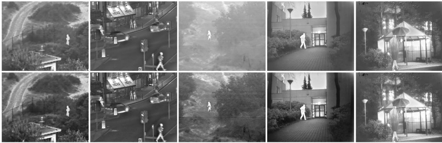
Fig. 8 Contrast enhancement of pre-fused image using Fast Guided Filter. The first row is the pre-fused image, and the second row is the final fused image after contrast enhancement
