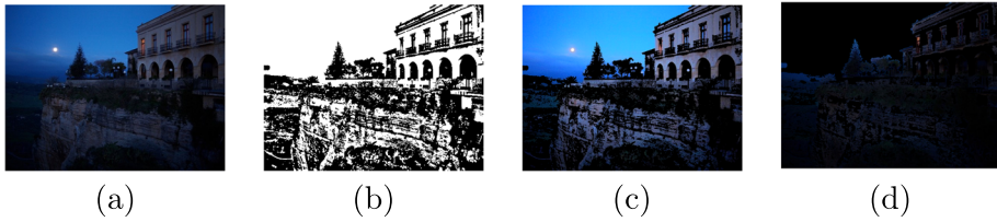
Fig. 2 Image segmentation method (a) input image, (b) fusion mask, (c) object region, (d) background region
