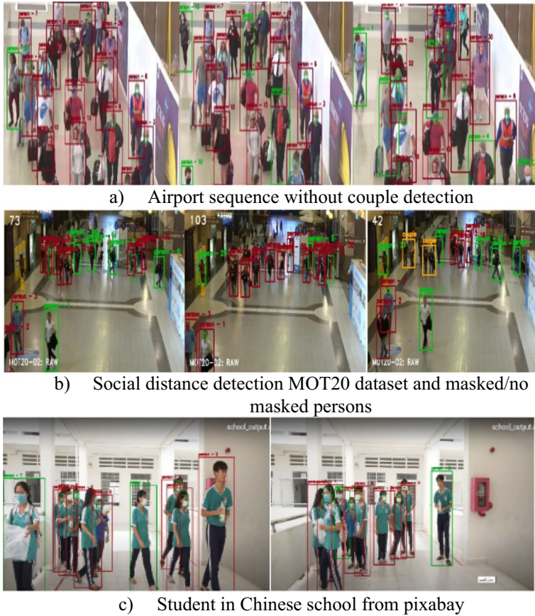
Fig. 16 Social-Scaled-YOLOv4&DeepSORT tested in outdoor a) Airport sequence without couple detection b) Social distance detection MOT20 dataset and masked/no masked persons c) Student in Chinese school from pixabay
