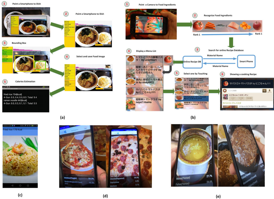
Fig. 2 Mobile applications for food analysis. (a) Kawano et al.’s app [50]. (b) Ingredients recognition and a cooking recipe recommendation [69]. (c) Calories estimation [113]. (d) Real-time mobile application classification on Pizza-Styles [29]. (e) Real-time mobile application classification on the GCC-30 data set [29]
