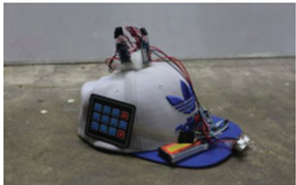
Fig. 17 Wearable cap for the indoor navigation system for blind people
