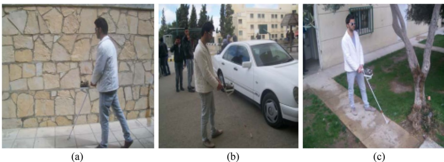
Fig. 22 Experimenting with the smart cane by a volunteer user (a) Identifying a wall by utilizing vibration and sound (b) Detecting barriers below the horizontal level of the smart cane (c) identifying barriers by turning the smart white cane right and left
