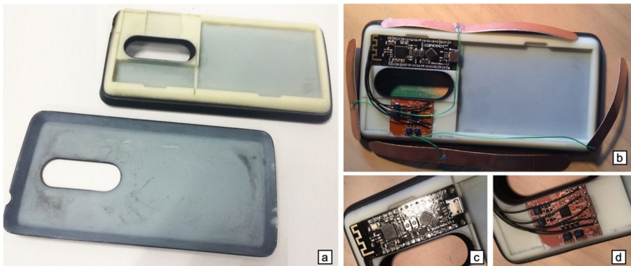
Fig. 2 The mobile phone case: (a) the front face and the rear face; (b) the capacitive sensing electrodes on the mobile phone case; (c) the flexible capacitive sensing board; (d) the Bluno Nano board served as micro-controller unit (MCU)
