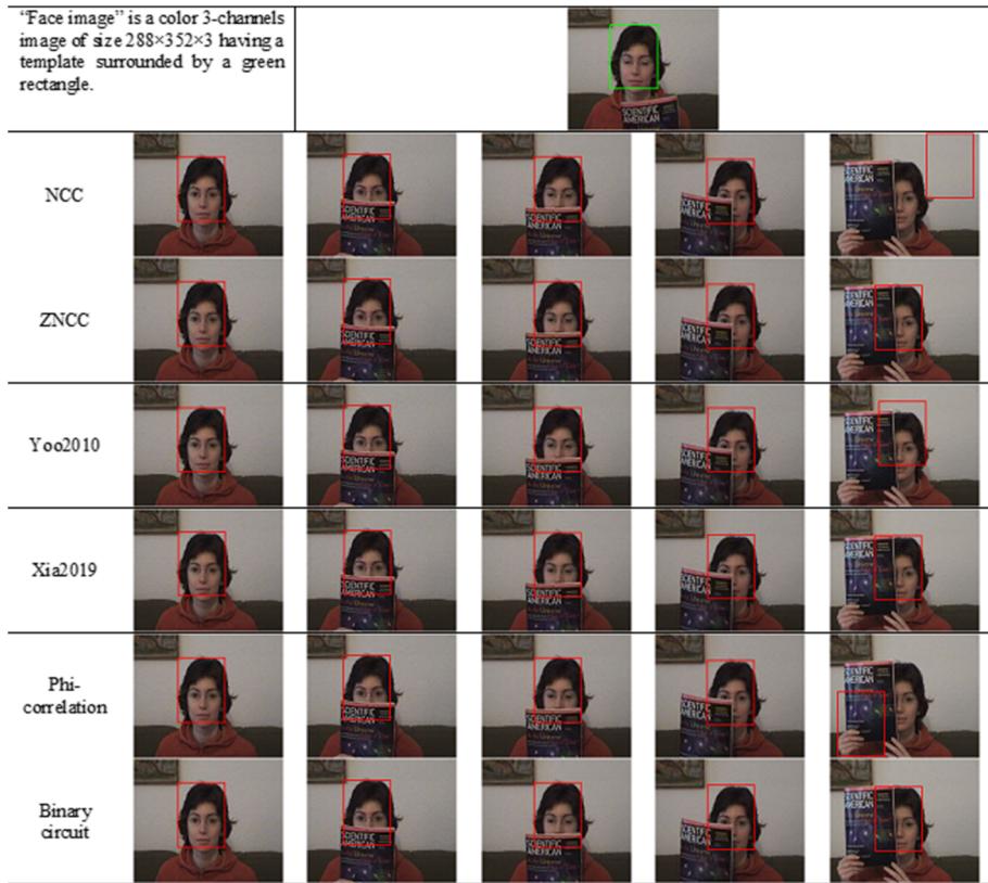
Fig. 12 Template matching results for different algorithms when applied to find corresponding locations in five different Face video frames. The first row shows the target template (outlined in green) in the initial frame of the video sequence. The second to seventh rows show the location of the target (outlined in red) identified by NCC, ZNCC, Yoo2010, Xia2019, \varphi -correlation, and Binary circuit, respectively
