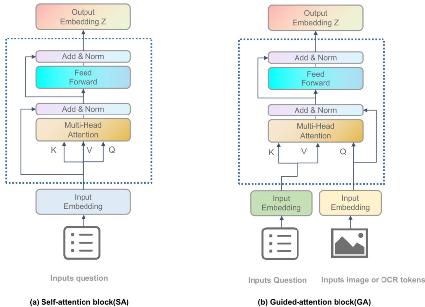
Fig. 3 Architecture of the two basic attention units
