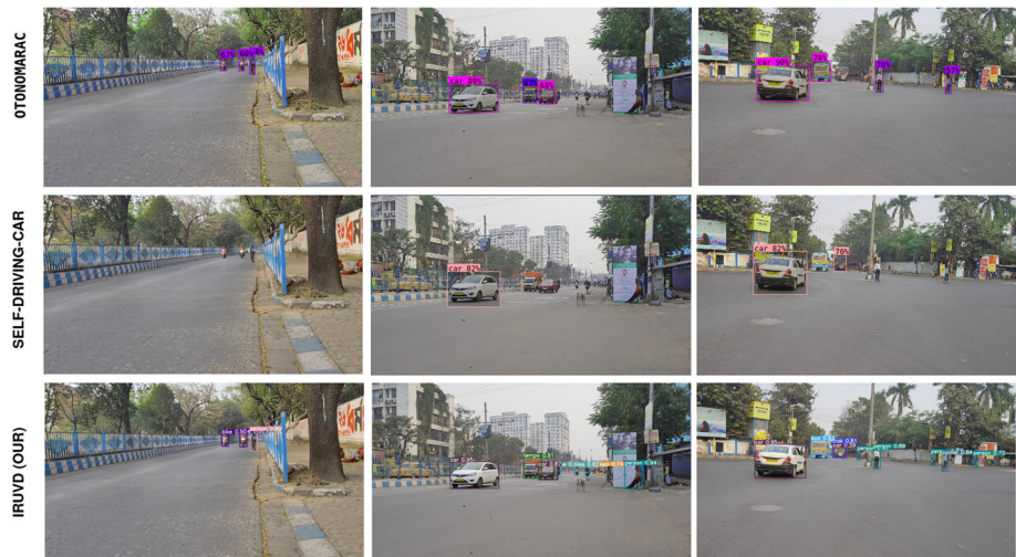
Fig. 19 Qualitative results of YOLOv5 model trained on Udacity Self-Driving-Car, Otonomarc and IRUVD (our) datasets
