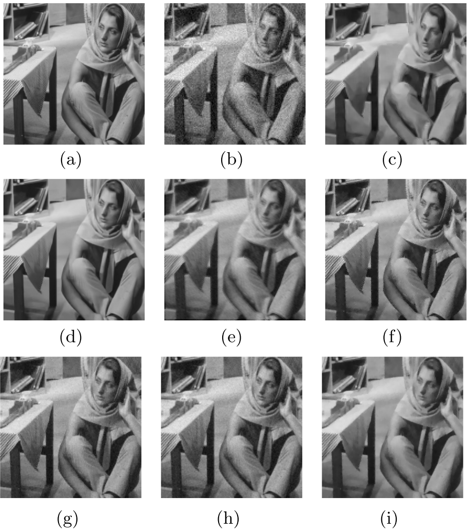
Fig. 3 Example image result (a), noisy image (b), Dual NLM Cauchy-Schwarz filter (c), BM3D filter (d), Bilateral filter (e), Wiener filter (f), Wavelet filter (g), Anisotropic diffusion filter (h) and Total Variation filter (i)
