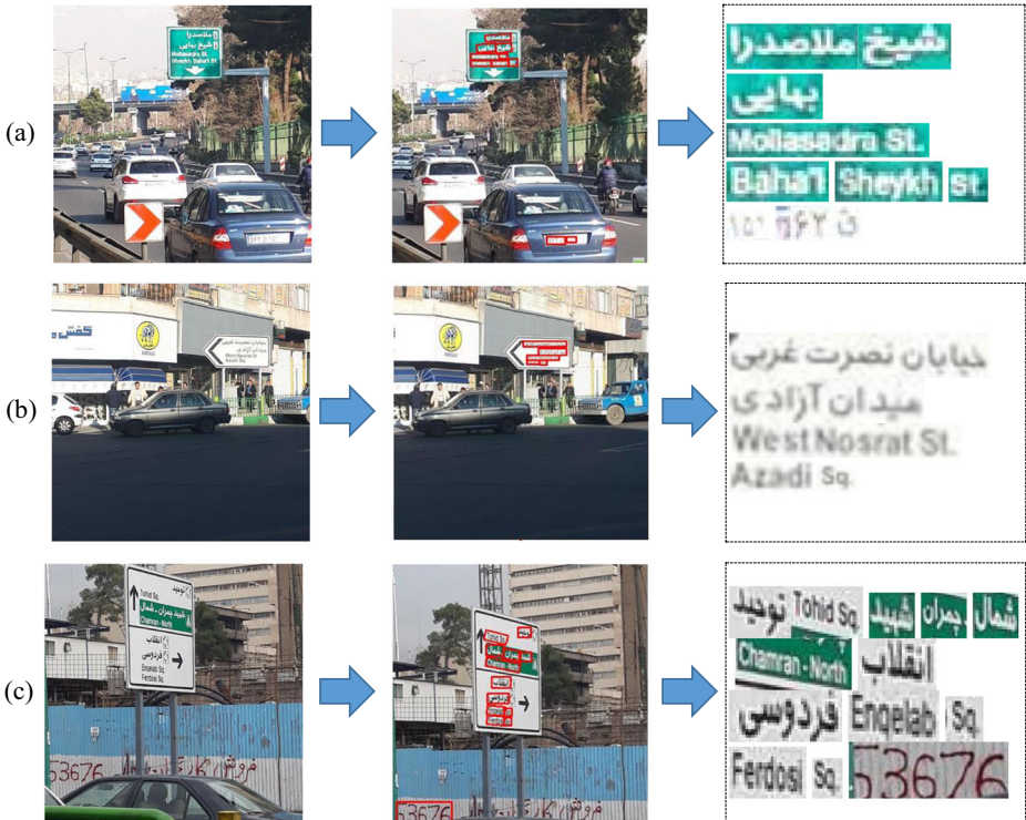
Fig. 4 The results of the CRAFT text detection model. (a) License plate detection, (b) Text detection; Scale challenge, and (c) Handwriting text detection and slant challenge
