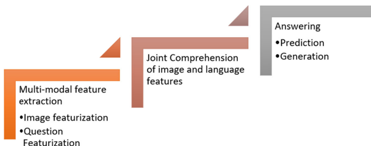
Fig. 1 Three phases of the general VQA pipeline
