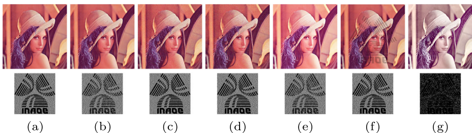
Fig. 8 Robust watermark results. Each column of the figure lists an attacked image and the obtained secret image using the extracted robust watermark (share) after different attacks were applied, i.e. JPEG compression 50% (a), blurring (b), Gaussian noise (c), salt & pepper noise (d), brighten (e), visible watermark adding (f) and tone mapping (g)
