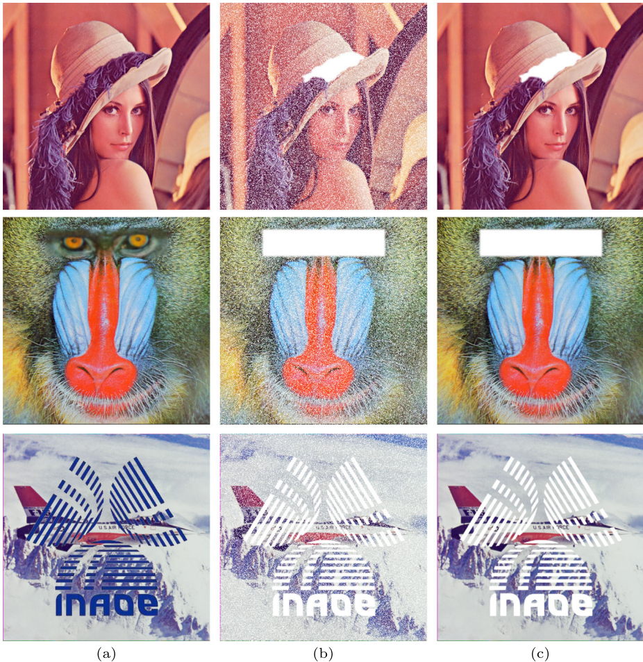
Fig. 9 Fragile watermark results. Attacked images with copy-move, blurring and collage attacks are shown in column (a) respectively. Authenticated images before filtering are listed in column (b). After filtering, authenticated images of column (c) are obtained
