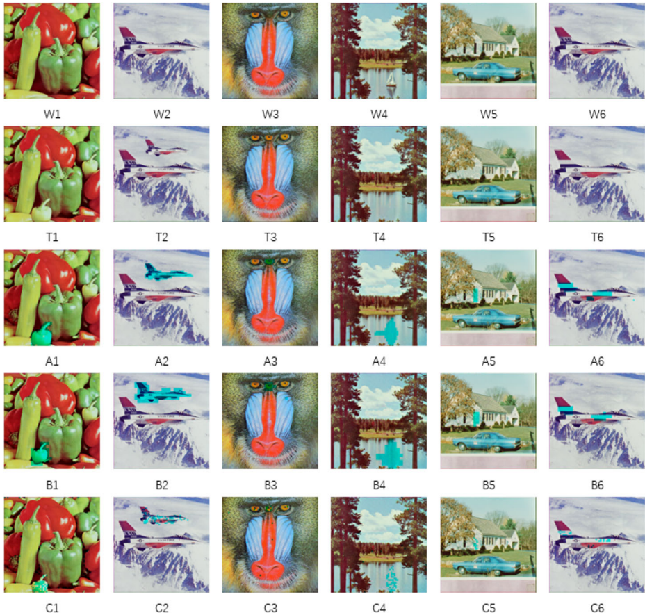
Fig. 17 Results of object attacks: (W1-W6) watermarked image (T1-T6) images after object attack: (T1) attacked image in “Peppers” by adding a new pepper, (T2) attacked image in “Airplane” by adding another airplane, (T3) attacked image in “Baboon” by adding an eye, (T4) attacked image in “Sail-boat” by removing the boat, (T5) attacked image in “House” by removing a window, and (T6) attacked image in “Airplane” by removing the “USA AIR FORCE”, and (A1-A6) tamper detection diagrams extracted from the proposed scheme, (B1-B6) tamper detection diagrams extracted from Duan et al.’s scheme [11], (C1-C6) tamper detection diagrams extracted from Kamili et al.’s scheme [9]
