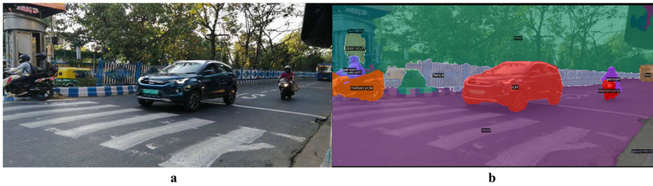
Fig. 28 Output images obtained after testing DETR-panoptic model our developed JUVDisi v1 database. a. input image, b. detr-output
