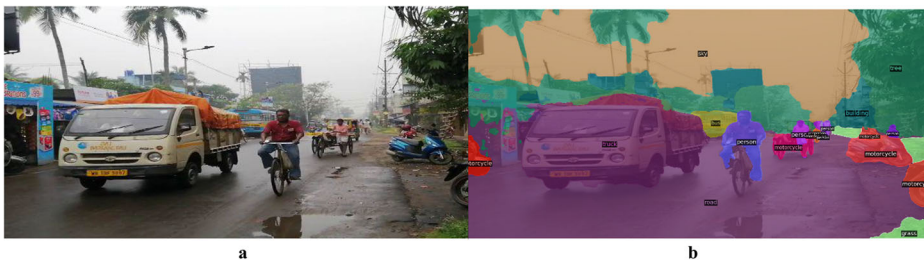
Fig. 29 Output images obtained after testing DETR-panoptic model our developed JUVDisi v1 database. a. input image, b. detr- output
