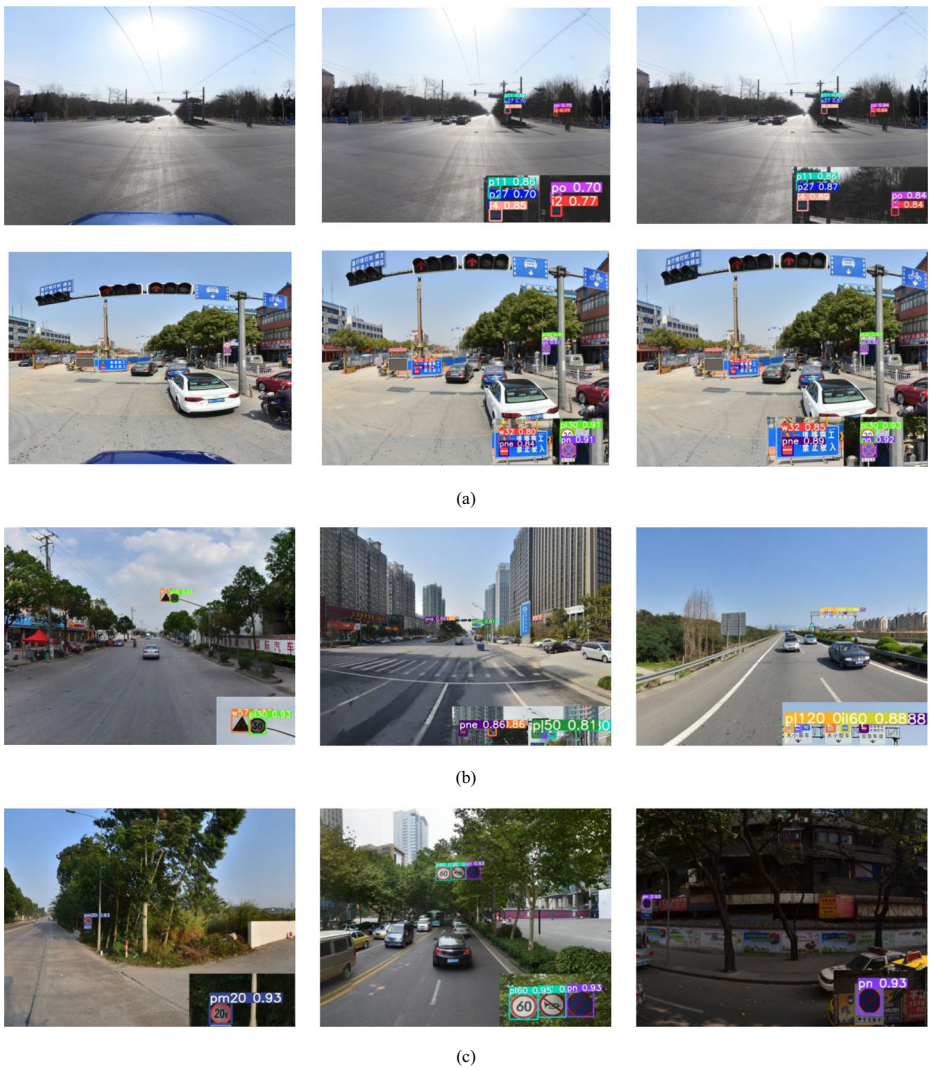
Fig. 11 Visualization results on the TT100K dataset: (a) detection results for YOLOv5-s and Ghost-YOLO; (b) detection results of the small target; (c) detection results in complex environments. Shadows, occlusions, cloudy, etc.
